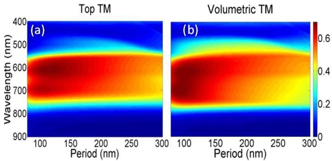
Fig. S1. Normalized absorptivity of the active layers as a function of periodicity ( $P$ ) of the silver grating under TM-polarized light. The absorption spectra are computed for varying  $P$  while keeping the same device parameters for  $w_1=50$  nm,  $w_2=30$  nm,  $LT_1=100$  nm,  $LT_2=20$  nm,  $LT_3=11$  nm,  $LT_4=4$  nm and  $LT_5=12$  nm.
