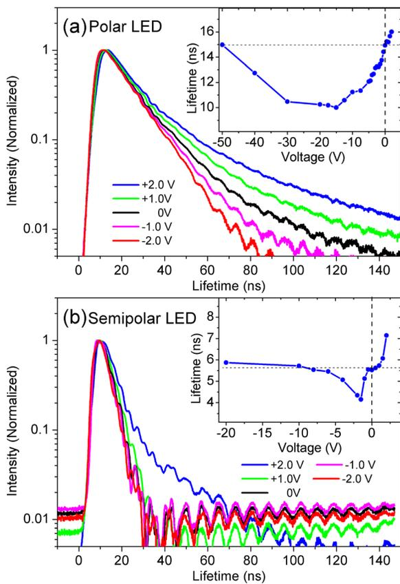
FIG. 3. TRPL spectra of (a) the polar LED device and (b) the semipolar LED device under external bias from  $-2$  to  $+2$  V. Inset shows the carrier lifetime (extracted using exponential fitting) for (a) the polar LED device under external bias from  $-50$  to  $+2$  V and (b) the semipolar LED device under external bias from  $-20$  to  $+2$  V.
