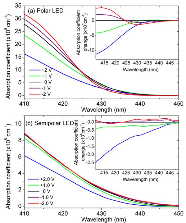
FIG. 4. Electroabsorption spectra of (a) the polar LED device and (b) the semipolar LED device under external voltage bias from  $-2.0$  to  $+2.0$  V. Inset: The absorption coefficient change compared to the zero bias condition.
