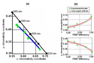
FIG. 1. (Color online) (a) Commission Internationale De L'Eclairage (CIE) chromaticity diagram for the tuning of chromaticity coordinates in our LbL spaced NC samples and (b) their semiempirical analytical model simulation results for color tuning based on FRET efficiency along with the experimental results.
