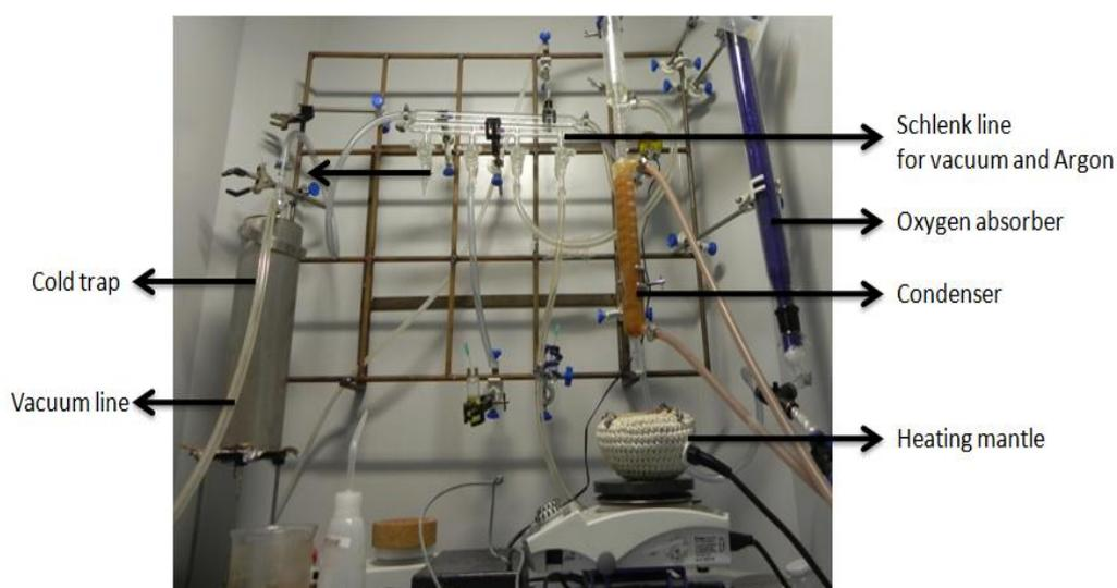
Figure 3.3.1 Synthesis set-up consisting of Schlenk line for Argon flow and vacuum. Cold trap is utilized for vacuum line. Oxygen absorber is utilized for making oxygen free Ar flow.
