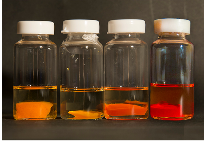
Figure 5.1: Our precipitated CdSe/CdSe 1-x Te x core/alloyed-crown NPLs in solution. They form gel-like structures.
