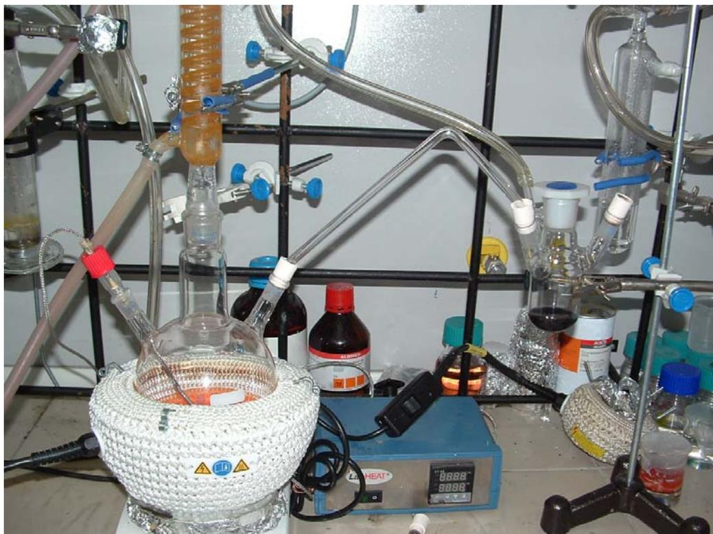
**Figure 3.2.1. A picture of CdTe nanocrystal synthesis setup. Precursors are produced in the main flask (left) and  $\text{Al}_2\text{Te}_3$  source is activated in the small three-necked flask (right).**
