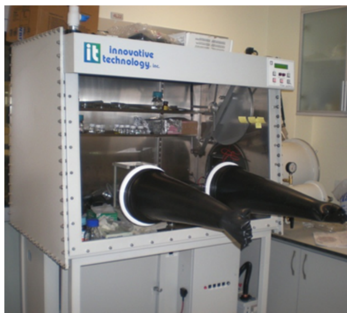
Figure 2.3: Glove box system to handle oxygen-sensitive chemicals.
