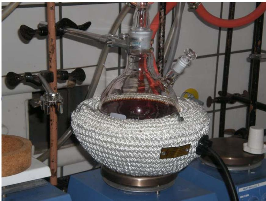
Figure 2.3.2 Red-brown mixture after the formation of CdTe nanocrystals (with our Phoremest collaborators).
