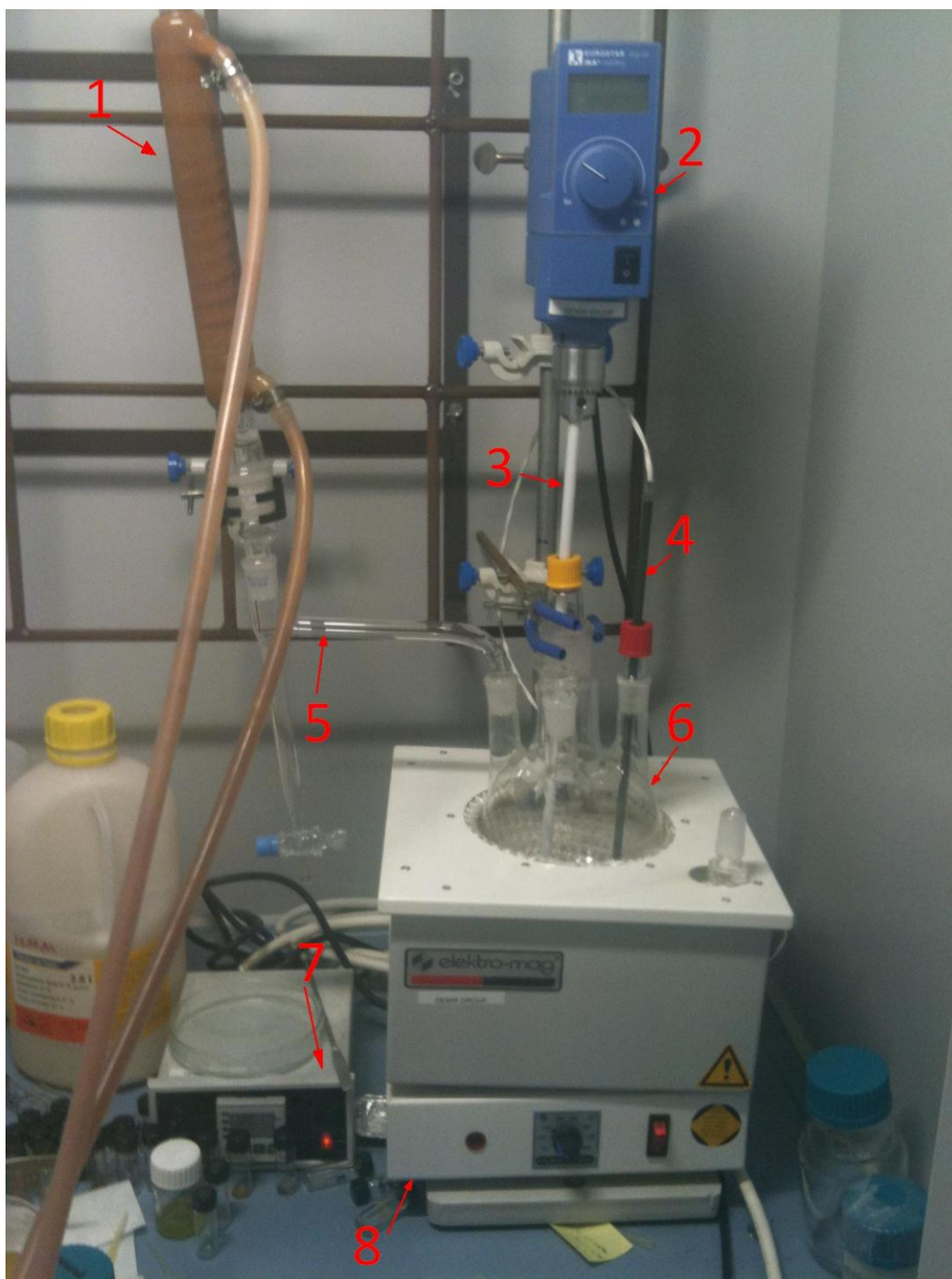
Figure 12. Our setup used for synthesizing sol-gel composites at UNAM.
