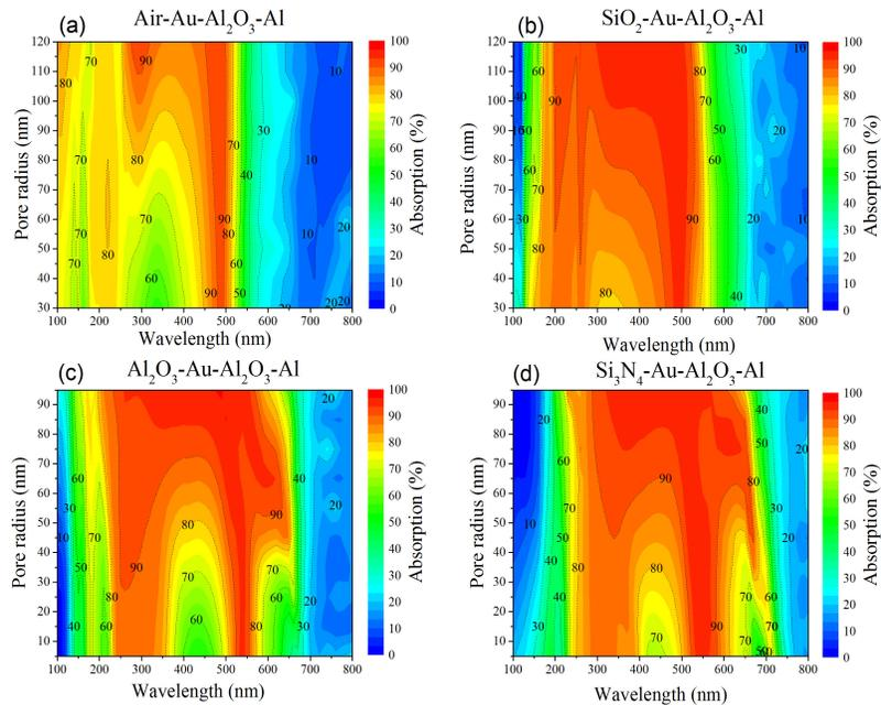
Fig. 5. Absorption profile of IMIM structure with top (a) *air*, (b) *SiO<sub>2</sub>*, (c) *Al<sub>2</sub>O<sub>3</sub>* and (d) *Si<sub>3</sub>N<sub>4</sub>* insulators versus pore radius and wavelength.
