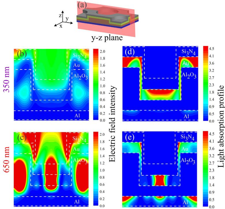
Fig. 6. Distribution of electric field intensity ( $|E|^2/|E_0|^2$ ) and light absorption profile ( $G/G_0$ ) in nanopatterned  $Si_3N_4$ - $Au$ - $Al_2O_3$ - $Al$  structure at the wavelengths of 350 and 650 nm. (a) Position of cross-section  $y$ - $z$  plane (red plane) in above mentioned structure. (b, c) Electric field intensity distribution for 350 and 650 nm along  $y$ - $z$  plane respectively. (d, e) Light absorption profile for 350 and 650 nm along  $y$ - $z$  plane respectively.
