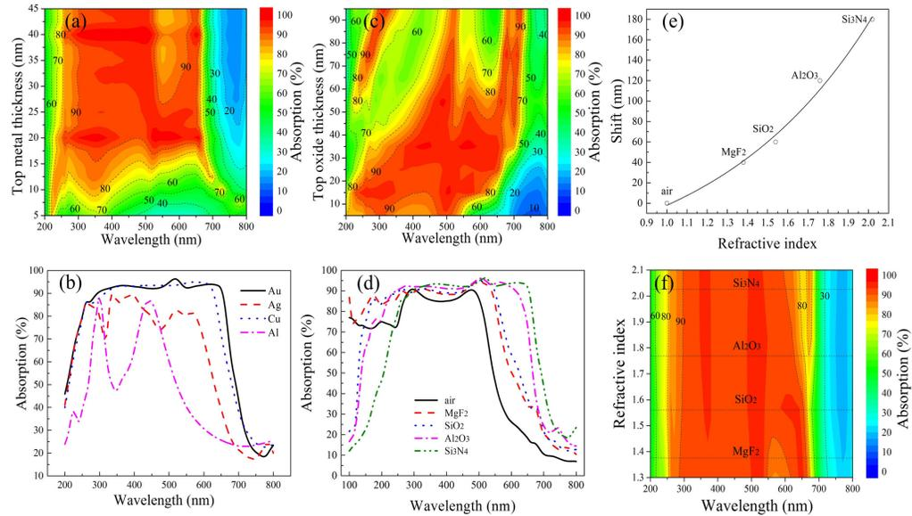
Fig. 3. Thickness and material type dependency on the absorption of the IMIM structure. (a) Dependence of top metal *Au* thickness. (b) Dependence of top metal material type. (c) Dependence of top insulator  $Si_3N_4$  thickness. (d) Dependence of different types of top insulator material. (e) Plasmon resonance shift versus refractive index of top insulator. (f) Dependence of different types of bottom insulator material.
