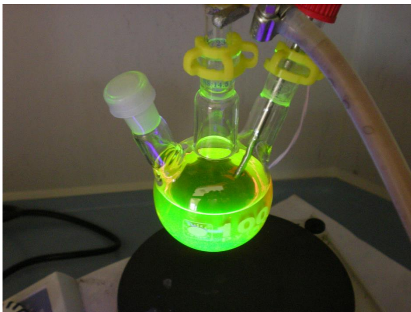
Figure 2.15. Exemplary photograph showing nonpolar CdSe/CdZnSeS/ZnS QDs synthesized in Demir Group synthesis laboratory.
