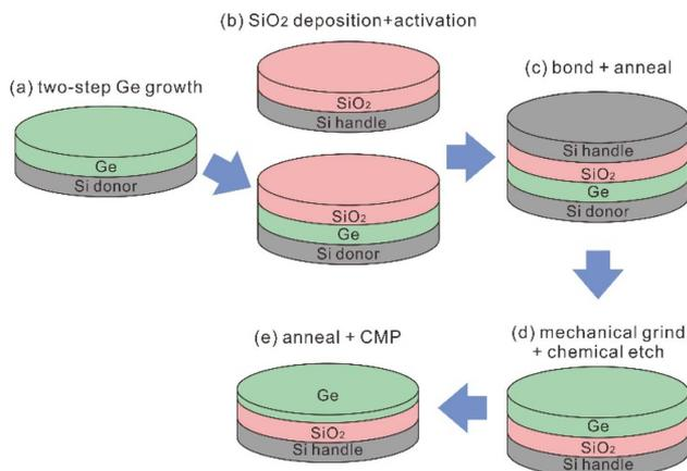
**Fig. 1.** Schematic flow of the fabrication of germanium-on-insulator (GOI) substrates with low threading dislocation density (TDD). All substrates are 200 mm in diameter.
