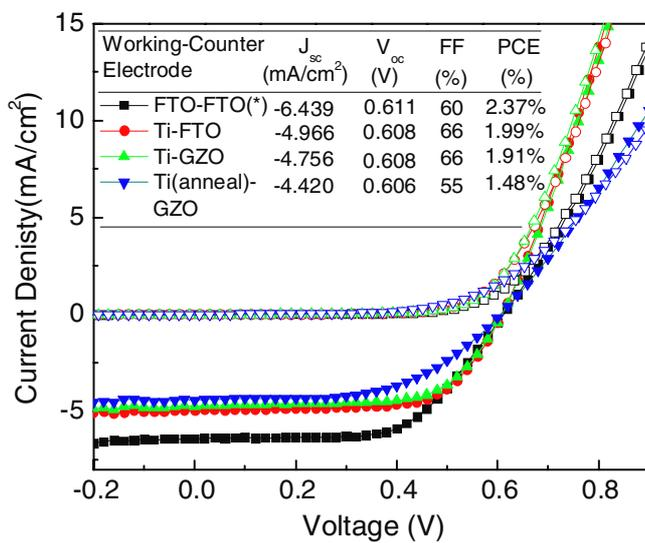
Figure 3.  $J$ - $V$  characteristics of the bottom- and top-illuminated DSCs under illumination (filled symbols) and in the dark (open symbols). Devices are named in the format of working electrode-counter electrode. (\*) denotes the bottom-illuminated device.
