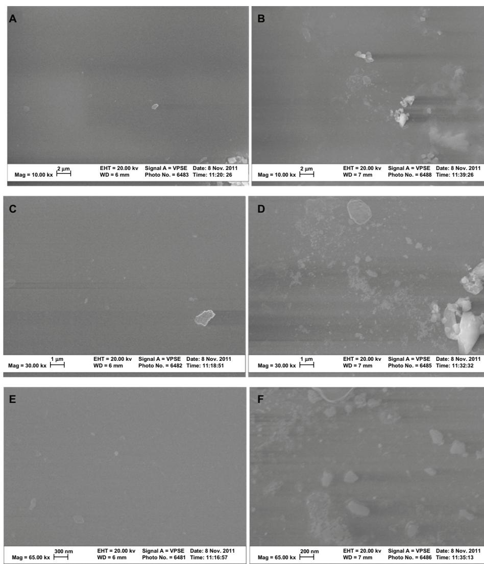
**Figure 2** SEM images of untreated PVC and NanoR PVC. Untreated PVC samples revealed a smooth surface (A, 10 KX; C, 30 KX; and E, 65 KX). On the other hand, NanoR PVC samples revealed a rough surface (B, 10 KX; D, 30 KX; and F, 65 KX).
