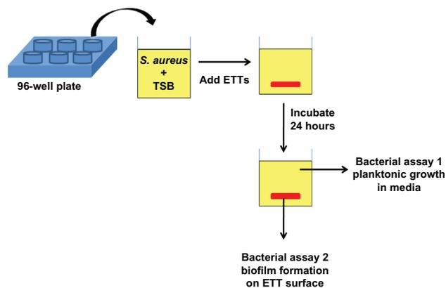
**Figure 1** Schematic of bacteria assays. Commercially available PVC ETTs were enzymatically degraded to create nanoscale surface roughness. Then, control PVC and NanoR ETTs were soaked into different concentrations of a fructose solution. Bacterial survival in the medium (assay 1) and biofilm formation on the ETT surfaces (assay 2) were quantified.
