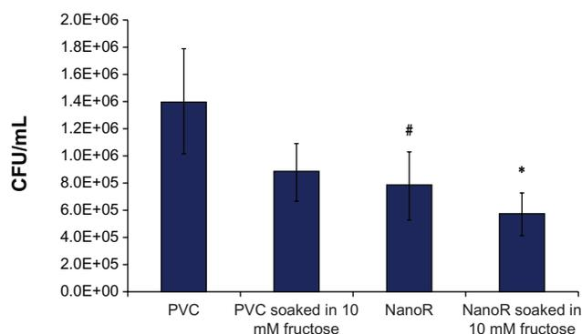
**Figure 5** *Staphylococcus aureus* colony counts on PVC and NanoR surfaces soaked in a 10 mM fructose solution. Biofilm formation decreased on NanoR and PVC surfaces soaked in a 10 mM fructose solution after 24 hours.
