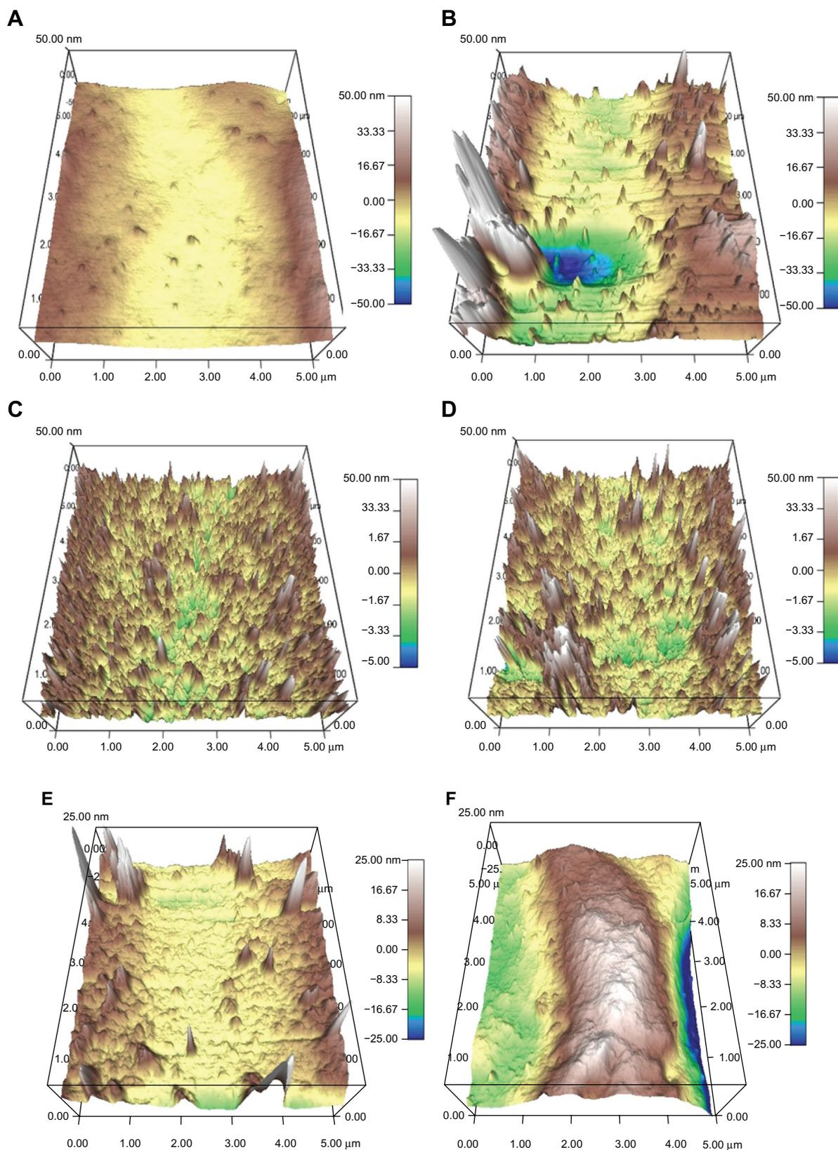
**Figure 3** AFM micrographs showing the topography of (A and B) control PVC and NanoR PVC; (C and E) control PVC soaked in 10 mM and 100 mM fructose; and (D and F) NanoR PVC soaked in 10 mM and 100 mM fructose, respectively. Micrographs revealed distinct differences in nanotopographies between the control PVC and NanoR PVC surface soaked in different metabolite concentrations.
