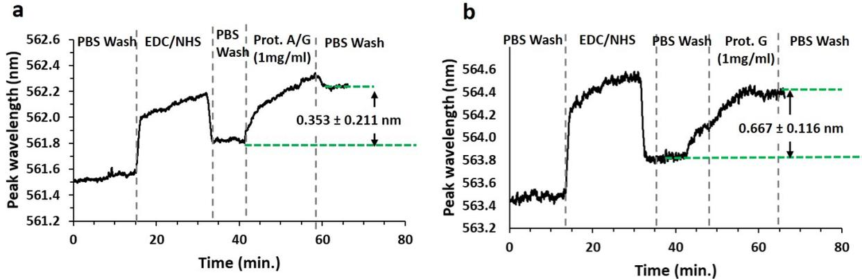
**Figure 3:** Real-time monitoring of surface sensitivity for monolayer protein A/G (a) and protein G (b) on DVD plasmonic surface.
