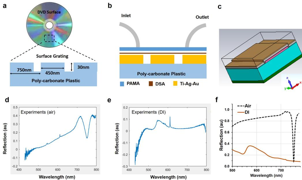
**Figure 1:** a. DVD surface grating. b. DVD microfluidic plasmonic sensor. c. Computation modeling of DVD sensor. d, e. Experimental plasmonic response of DVD surface with air and DI medium. f. Computational result of DVD surface with air and DI medium.
