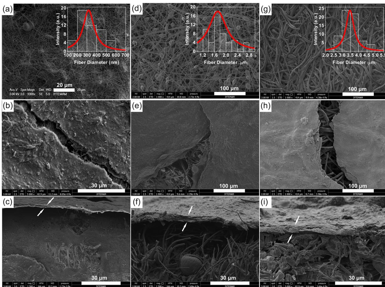
**Figure 1.** SEM images of polymer nanofibers: (a) PVDF nanofiber and PVDF-MWCNT, (b) top view and (c) side view; (d) PS nanofiber and PS-MWCNT, (e) top view and (f) side view; (g) PMMA nanofiber and PMMA-MWCNT, (h) top view and (i) side view. Insets in a, d, and g show the distribution of fiber diameter.
