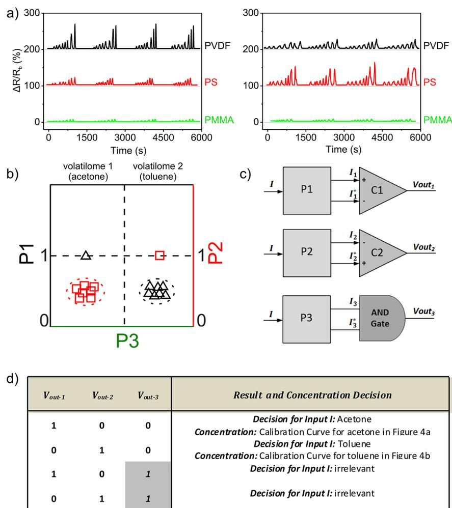
**Figure 6.** (a) Volatilome responses of the sensing microchannels with increasing acetone concentrations (left) and toluene concentrations (right). (b) Normalized response of sensing microchannels P1, P2, and P3 upon input  $I_1$ ,  $I_2^*$  and  $I_1^*$ ,  $I_2$ . (c) Hardware setup for volatilome analyzer (Cx: Comparator 1 and 2; P1, P2, and P3: sensing microchannels). (d) Decision table for volatilome recognition.
