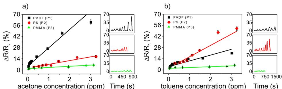
**Figure 4.** (a) Concentration-dependent acetone responses of PVDF (P1), PS (P2), and PMMA (P3). (b) Concentration dependent toluene responses of PVDF (P1), PS (P2), and PMMA (P3). The inset graphs in a and b show the concentration-dependent real-time responses of P1, P2, and P3 for acetone and toluene.
