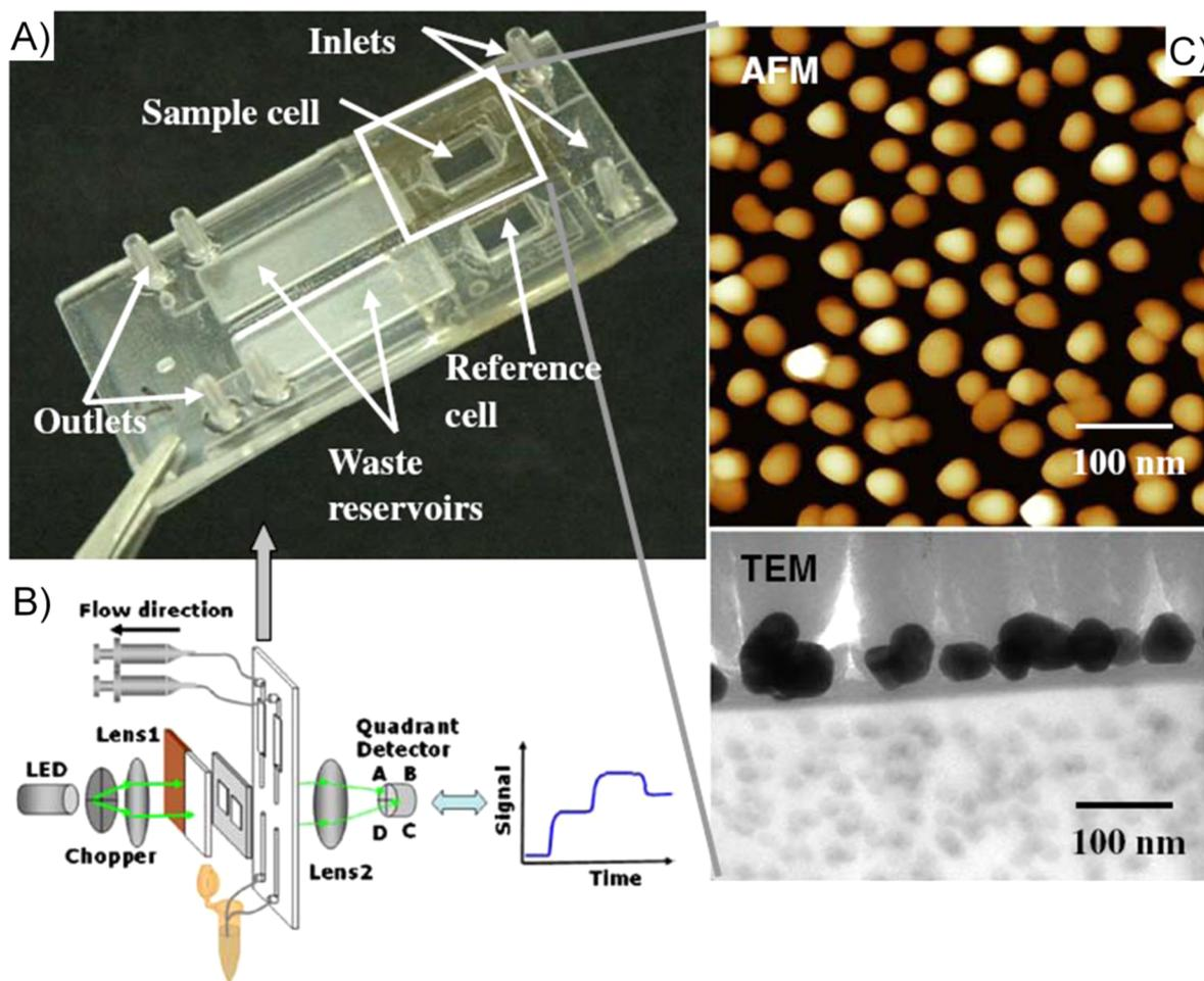
**Figure 10.** A microfluidic-based LSPR system. (A) The gold-nanosphere-coated LSPR channel and the control channel are positioned next to each other in the photograph of the microchip. (B) The experimental schematic indicating the LED light source, microfluidic chip, and photodetector. (C) Atomic force microscopy (AFM) and transmission electron microscopy (TEM) images of the nanoparticles on the chip. Reprinted with permission from ref 194. Copyright 2009 Springer.
