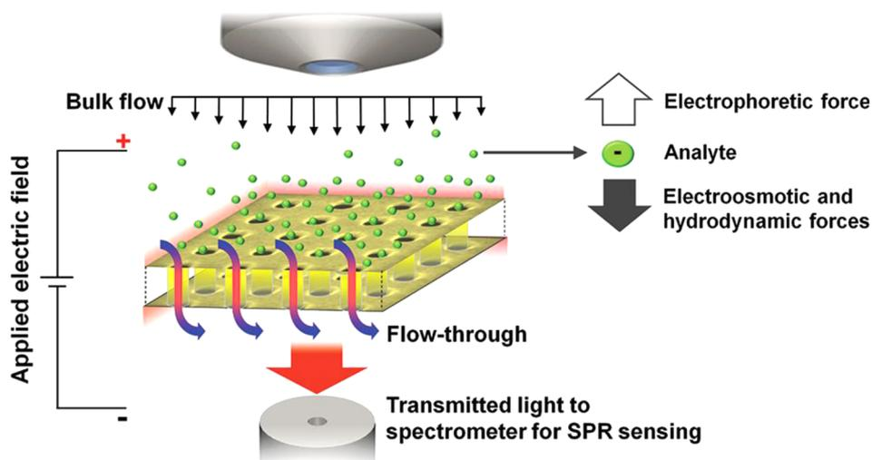
**Figure 6.** A nanohole array integrated with fluidics. The flow-through plasmonic nanostructure enabled local concentration of analytes. The method presented 100-fold concentration and simultaneous sensing of a protein. Further, the method presented 10-fold improvement in sensing speed in comparison to the control experiment with no analyte concentration. Reprinted with permission from ref 101a. Copyright 2012 American Chemical Society.
