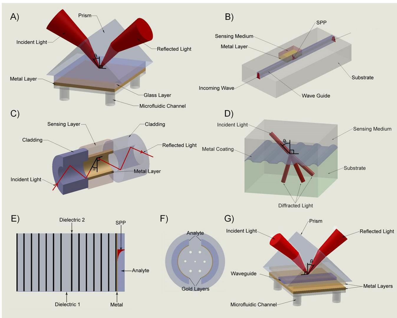
**Figure 4.** Most common surface plasmon operation modes for light coupling: (A) Kretschmann configuration for prism coupling, (B) waveguide coupling, (C) fiber-optic based coupling, (D) grating coupling, (E) planar waveguide photonic crystal coupling, (F) honeycomb photonic crystal coupling, (G) waveguide-based coupling in Kretschmann configuration.
