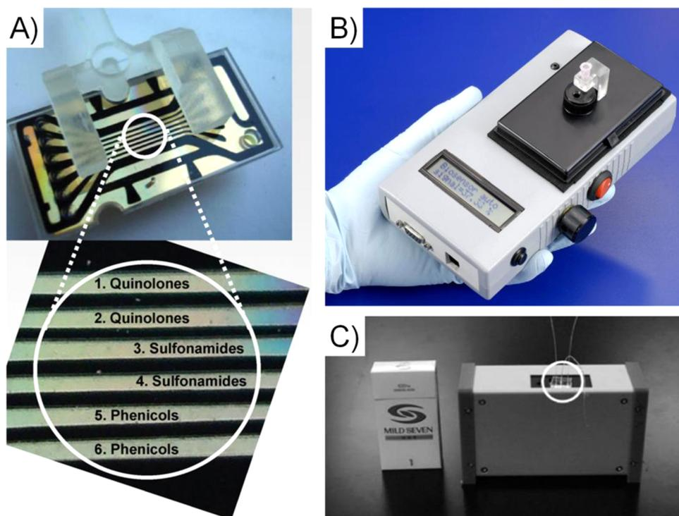
**Figure 8.** Portable SPR biosensor platforms. (A) A multichannel cartridge to be used for on-site antibiotic detection in milk samples. Reprinted with permission from ref 171. Copyright 2010 Elsevier. (B) Portable SPR biosensor prototype to be used with microfluidic chips. Reprinted with permission from ref 172. Copyright 2009 Elsevier. (C) Portable microfluidic-based device for cardiac marker detection. Reprinted with permission from ref 173. Copyright 2006 American Chemical Society.
