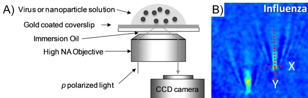
**Figure 14.** SPRi system used for individual virus particle imaging. (A) The schematic for the SPRi experiment utilizing an objective in the Kretschmann configuration and an inverted microscope. (B) SPR images of the influenza A virus in PBS buffer. Reprinted with permission from ref 218. Copyright 2010 National Academy of Sciences.
