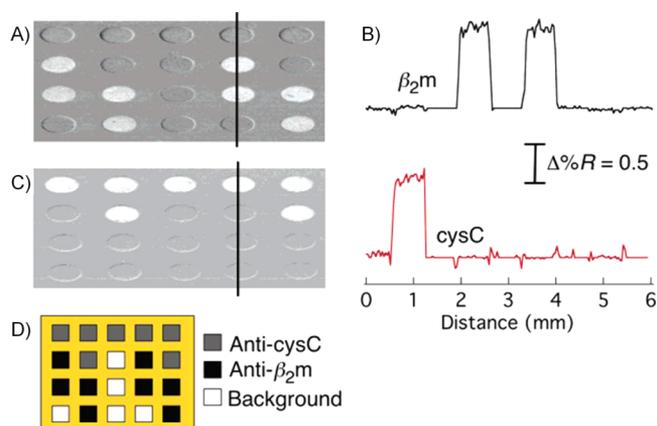
**Figure 11.** SPRi detection of 50 nM  $\beta_2$ -microglobulin ( $\beta_2\text{m}$ ) and 100 nM cystatin C (cysC). (A and C) Images for  $\beta_2\text{m}$  and cysC detection, respectively. (B) The line profiles indicated in parts A and C show signal only in the corresponding channels where the antibodies were positioned. (D) Map of the antibodies and control channels used in parts A and C. Reprinted with permission from ref 214. Copyright 2006 American Chemical Society.
