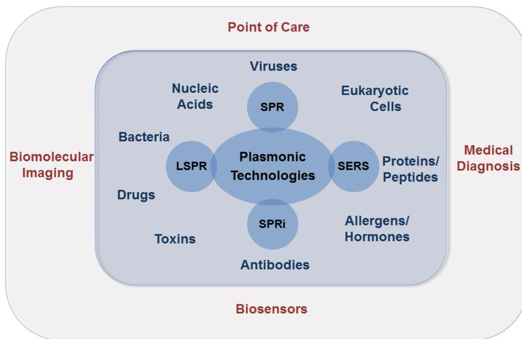
**Figure 1.** Plasmonic-based technologies for versatile biosensor applications. SPR stands for surface plasmon resonance, LSPR for localized surface plasmon resonance, SPRi for surface plasmon resonance imaging, and SERS for surface-enhanced Raman scattering.
