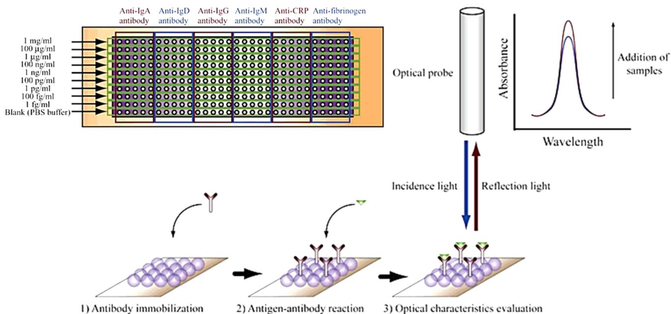
**Figure 9.** The distribution of six different antibodies corresponding to nine concentrations from 1 fg/mL to 1 mg/mL is shown along with the reflection-mode, intensity-based LSPR detection method. Reprinted with permission from ref 193. Copyright 2006 American Chemical Society.
