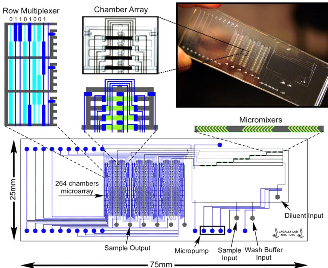
**Figure 13.** Layout of the element addressable microdevice for SPRi experiments, depicting the 264 chamber microarray, accessed by various features, such as a micropump, microvalves, micromixers, input/output channels, and a row multiplexer. A detailed microarray is shown along the photograph of the microfluidic chip. Figures are courtesy of Prof. Eric T. Lagally.
