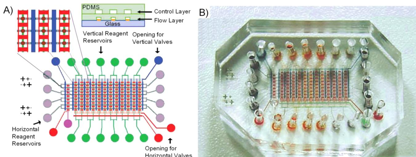
**Figure 12.** A microfluidic-based SPRi platform. (A) Schematic of the microchip for the SPRi experiment. The lower layer is where the immunoreactions take place, and the upper layer controls the fluid flow by microfluidic pumps. (B) The microfluidic device with dyed fluids to illustrate the microchannels. Figures are courtesy of Prof. Richard N. Zare.
