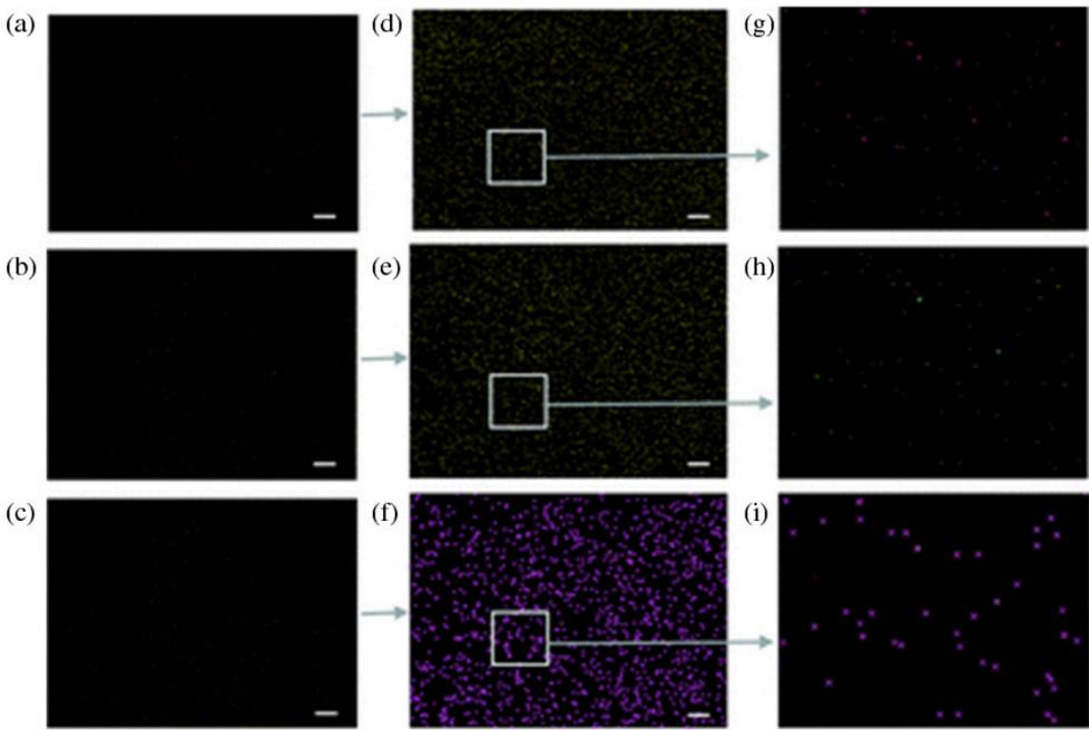
**Fig. 3.** Fluorescence imaging of CD4<sup>+</sup> T lymphocytes on a microchip.<sup>36</sup> The captured CD4<sup>+</sup> T lymphocytes were stained AF488-anti CD3 (a) and AF647-anti CD4 (b). To facilitate rapid counting, fluorescence images were merged for better recognition by a counting algorithm (c). Images (d)–(f) were processed and counted by the counting algorithm. Images (g)–(i) are the corresponding portions that were shown in images of (d)–(f), respectively.
