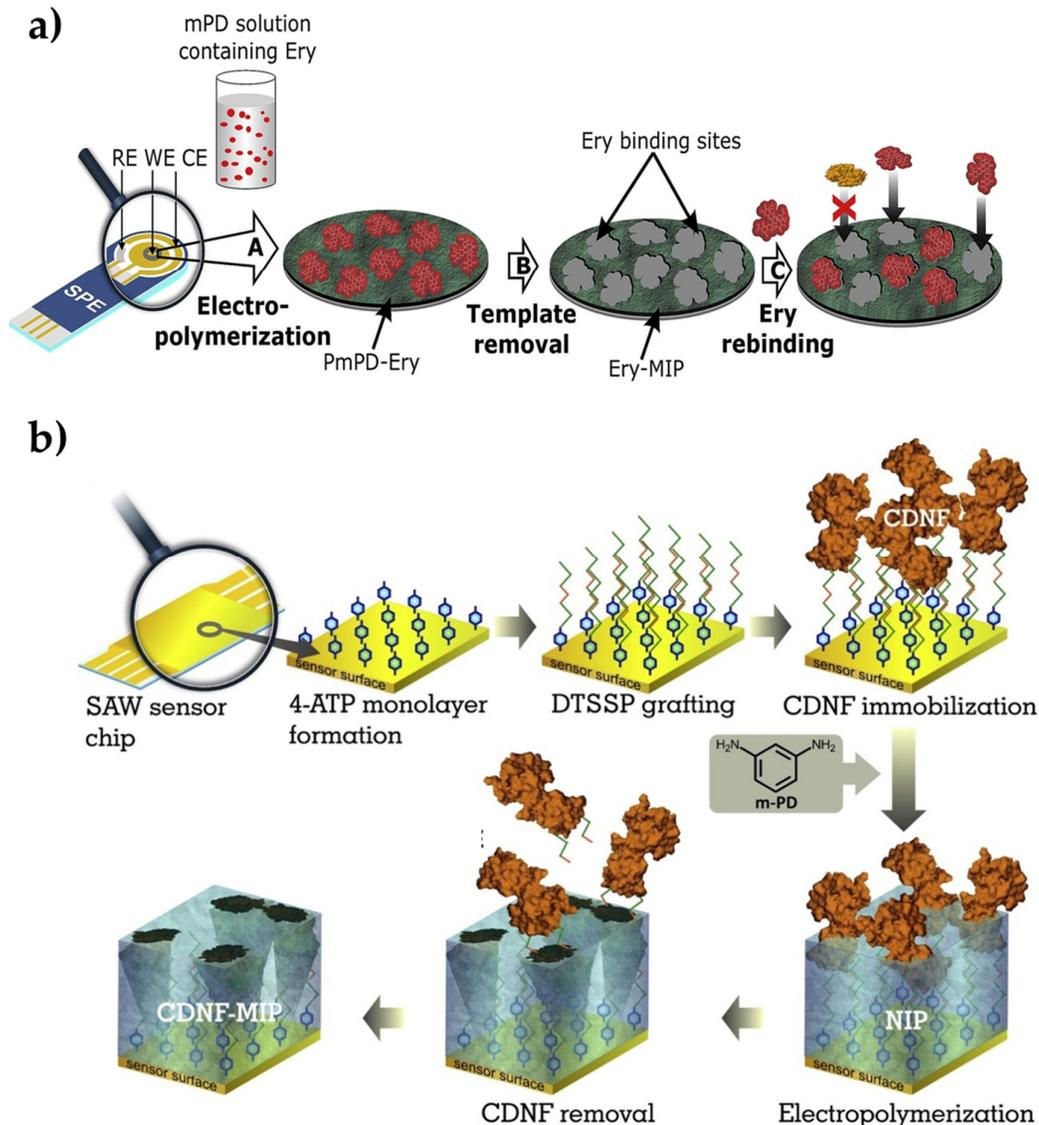
**Figure 3.** Preparation of the erythromycin-imprinted electrochemical sensor (a) and cerebral dopamine neurotrophic factor protein-imprinted surface acoustic wave sensor (b). Republished with permission from Ayankojo et al. and Kidakova et al. [87,88].
