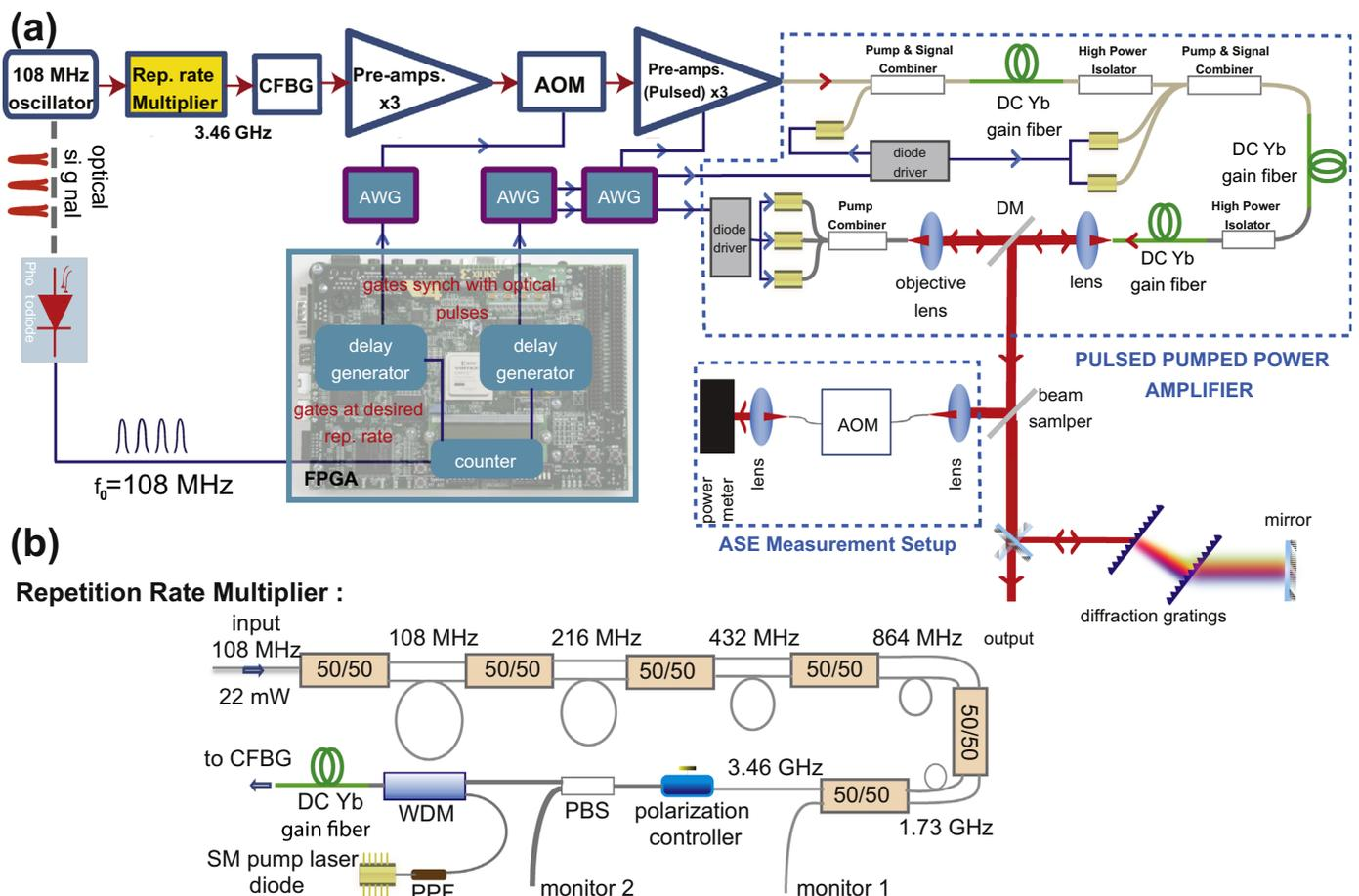
**Fig. 1.** (a) Schematic diagram of the experimental setup. CFBG: chirped fiber Bragg grating, AOM: acousto-optic modulator, AWG: arbitrary waveform generator, FPGA: field programmable gate array, DM: dichroic mirror, WDM: wavelength division multiplexer, PBS: polarizing beam splitter, PPF: pump protection filter, SM: single-mode, DC: double-clad. (b) Schematic setup of high repetition rate multiplier followed by first stage fiber amplifier.
