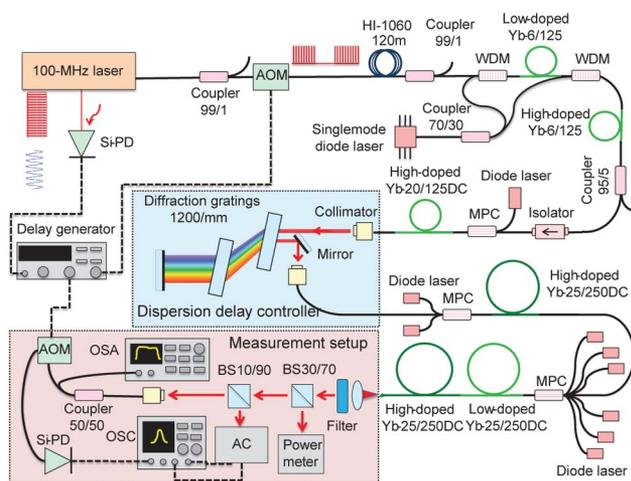
**Fig. 1.** Schematic diagram of the setup. AOM, acousto-optic modulator; WDM, wavelength-division multiplexer; MPC, multiple pump-signal combiner; Si-PD, silicon photodetector; AC, autocorrelator; OSA, optical spectrum analyzer; OSC, oscilloscope.
