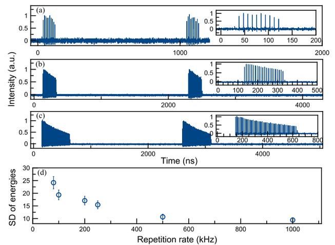
**Fig. 2.** Measured temporal profile of the pulse burst at 50 W output power. Inset: close-up showing the pulse train at repetition rates of (a) 1 MHz, (b) 500 kHz, and (c) 200 kHz. (d) Standard deviation (SD) of pulse energies within the pulse bursts as a function of burst repetition rate measured at 50 W.
