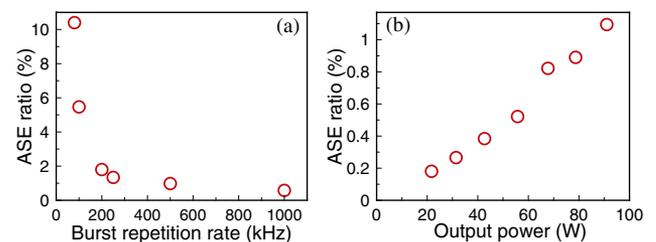
**Fig. 3.** (a) Measured ASE/output power ratio as a function of burst repetition rate at 50 W output. (b) Measured ASE/output power ratio versus output power, for which the burst repetition rate was kept at 1 MHz.
